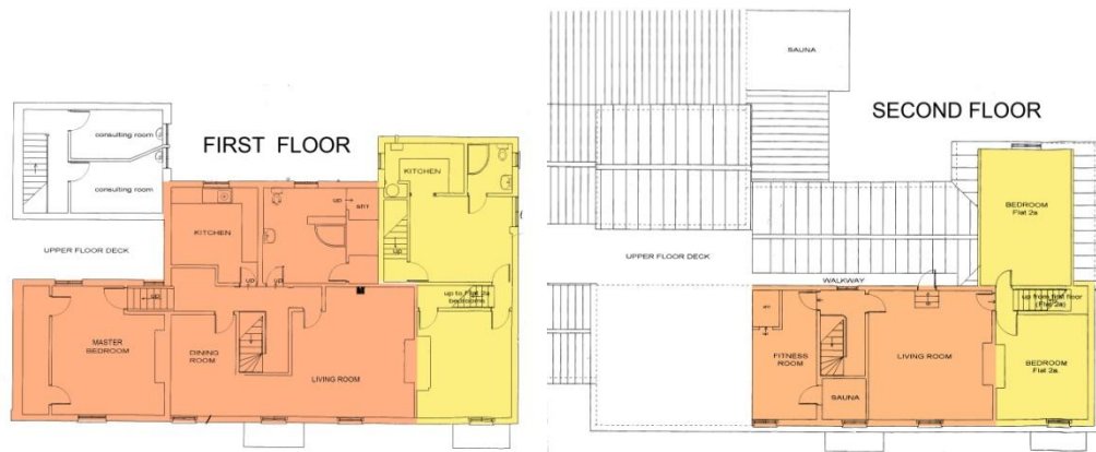
First and second floor plans showing the division of the property into Flats 2a and 2b.
